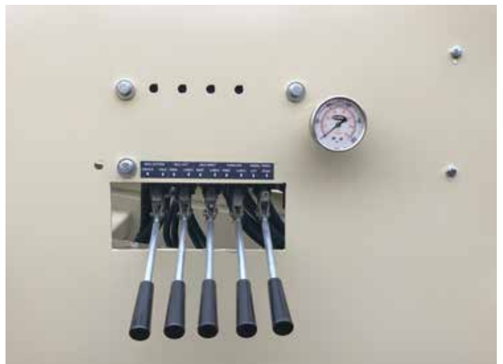
10/ HYDRAULIC CONTROL CENTER
